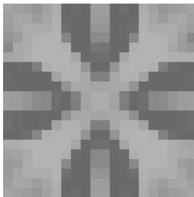
Fig. 4. Stress constrained design for maximum torsional rigidity.
